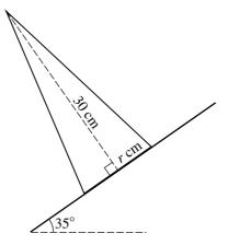
A uniform solid cone has height 30 cm and base radius r cm. The cone is placed with its axis vertical on a rough horizontal plane. The plane is slowly tilted and the cone remains in equilibrium until the angle of inclination of the plane reaches  $35^{\circ}$ , when the cone topples. The diagram shows a cross-section of the cone.
